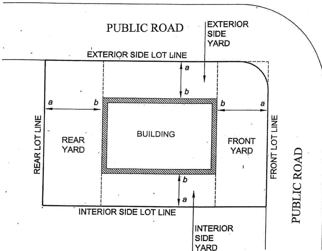
DISTANCE  $ab$  REPRESENTS THE SHORTEST DISTANCE MEASURED BETWEEN THE LOT LINE AND THE NEAREST PART OF THE MAIN BUILDING. DISTANCE  $ab$  MUST BE A MINIMUM OF THE REQUIRED YARD SPECIFIED IN THE BY-LAW
