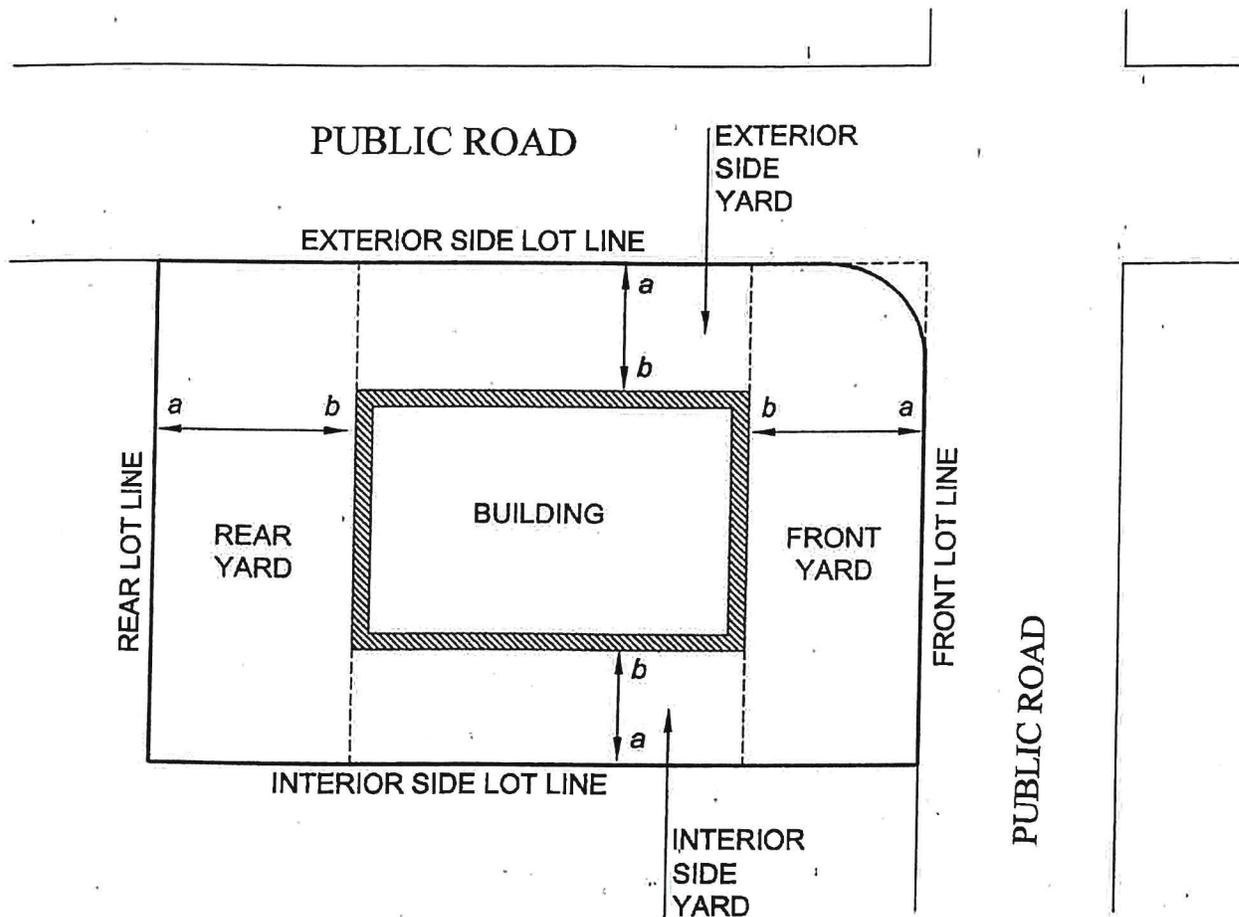
DISTANCE *ab* REPRESENTS THE SHORTEST DISTANCE MEASURED BETWEEN THE LOT LINE AND THE NEAREST PART OF THE MAIN BUILDING. DISTANCE *ab* MUST BE A MINIMUM OF THE REQUIRED YARD SPECIFIED IN THE BY-LAW
